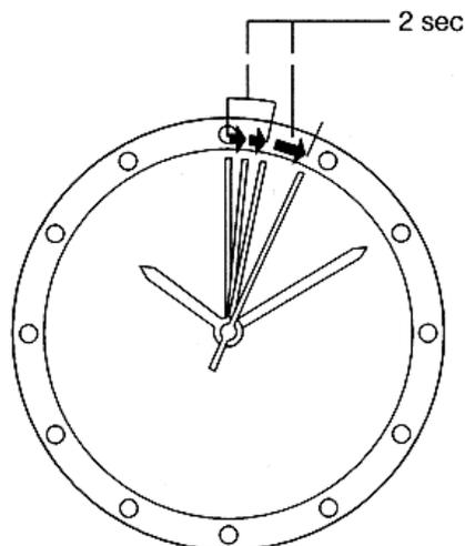
If the watch stops, subsequent exposure to light allows the 'quick start' function to start again, and the second hand moves with a hitch to indicate that the time is incorrect.
