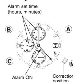
Press button **(M)** to switch to the alarm 2 (AL-2) mode.
