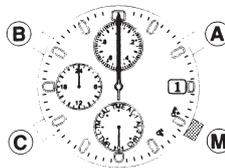
1. Press button (M) to switch the watch to the 0-position check mode (▶0◀). The hour hand, minute hand, 24H hand, second hand, date and function hand will advance rapidly to the 0-position (base position).
