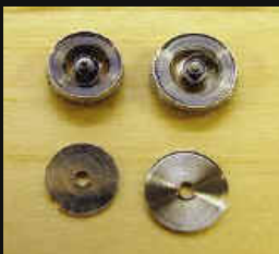
barrel – spring wrapped – center is arbor – barrel cap
