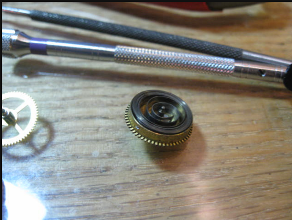
OLD BLUED STEEL MAIN REMOVED NEW STEEL MAIN INSTALLED
