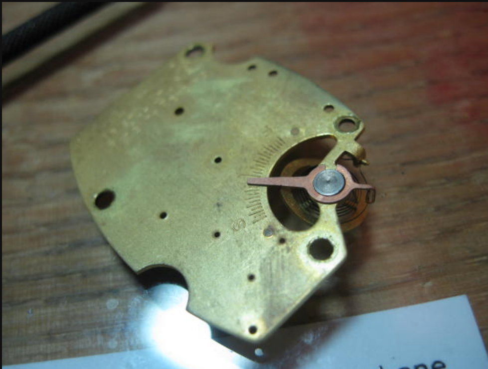
REMOVED RUSTED HAIR SPRING REPLACED WITH NEW ADAPTED
