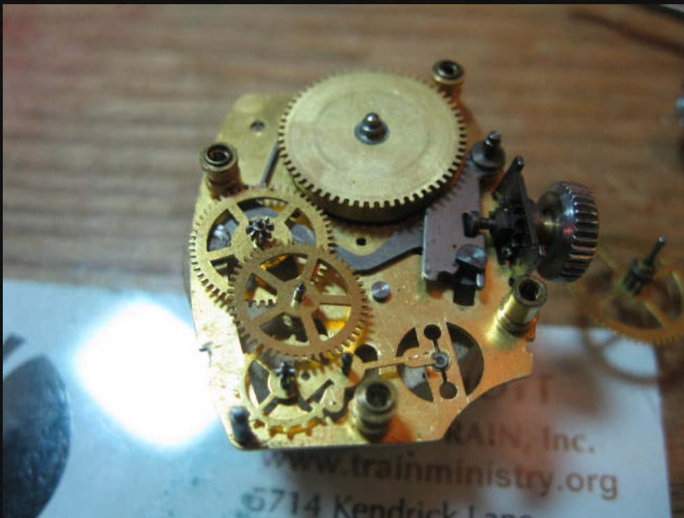
BARREL AND ARBOR INSTALLED
