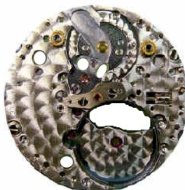
LIFT OUT MAIN SPRING BARREL
